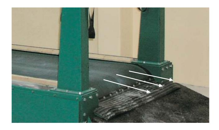
The rear end of Haico treadmill has designed so that dung is quided handily away from the belt. This makes easier the daily cleaning and keeps the inside of the treadmill more clean and more .hygiene
