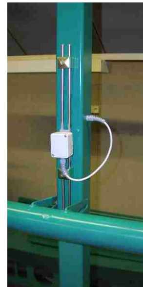
Heart rate receiver receives the rate signal and sends it to the display
