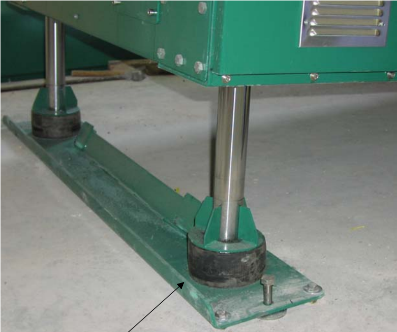
Vibration absorbers in the front of the frame
