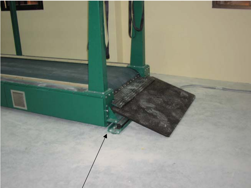
Vibration absorbers at the back of the frame
