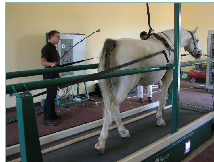
Pulling belts are connected to the safety harness and the pulling force can be steplesly adjusted between 0 to 85 kg (850N) manually or automatically via the test programs.
